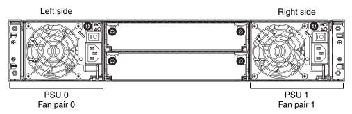
Figure 3-1 Location of Fan and Power Supply Units (PSUs)
